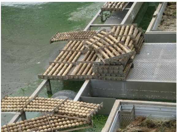
Contamination of photocatalyst balls
