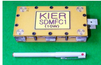
1998 10W DMFC stack for portable application
