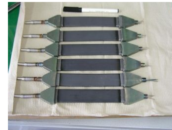
1kW flat tubular and tubular SOFC stack
