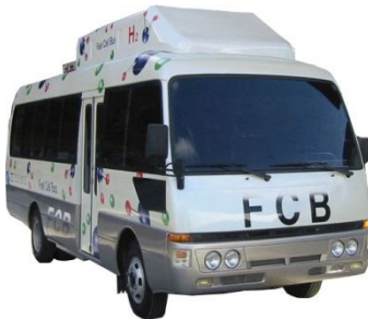
2006 Fuel Cell/Battery Hybrid mini-Bus with a 50kW Stack Module
