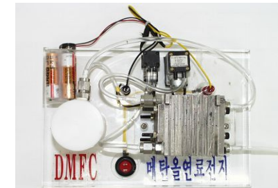
2000 15W DMFC system for portable application
