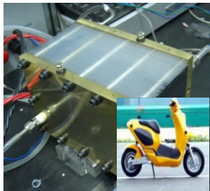
2007-2009 DMFC/Battery Hybrid scooter with a 500W Stack Module
