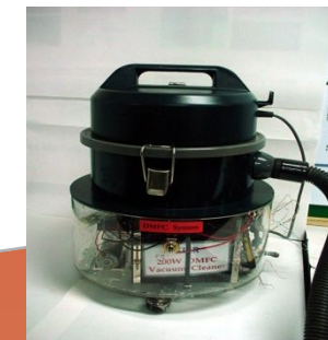
2002-2004 100W DMFC/Battery hybrid sys. for vacuum cleaner
