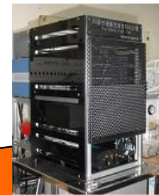
1999-2004 1kW PEMFC system for Small & Portable Application
