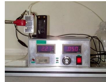
1999 3W DMFC system for a cellular phone
