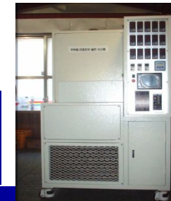
1999-2001 5kW PEMFC system for RPG with Natural Gas reformer
