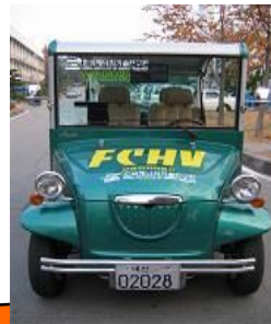
2004 Fuel Cell/Battery Hybrid Vehicle with 2kW Air-cooled Stack
