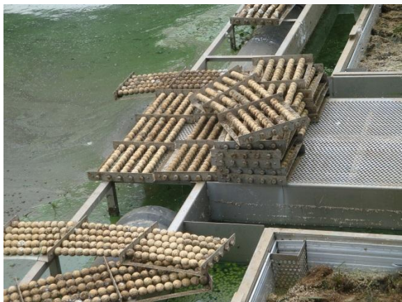
Contamination of photocatalyst balls
