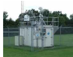
PM2.5 Chemical Composition On-line measurement(Ion, Carbon, Metal)
